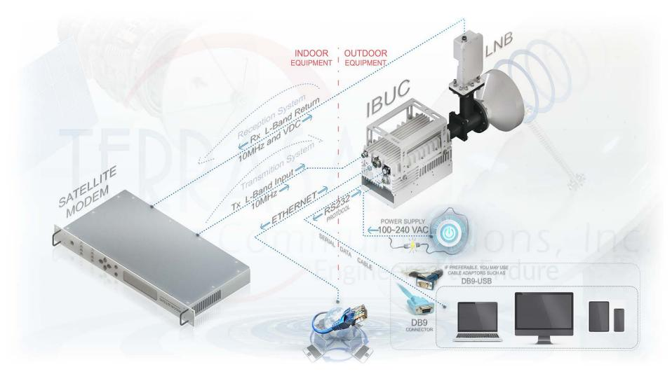
Figure 2.11 AC Power IBUC System Configuration
