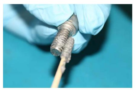
Figure 3.8 Applying the Anti-Seize Lubricant
